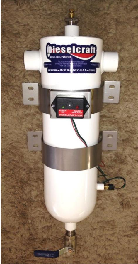
The poly bag containing fittings will have the Megaloc Sealant, a reducing bushing with a bleeder valve installed for the top of the separator, a ball valve for the bottom and one pipe plugs. The 1/8 NPT pipe plug is intended for the sensor port if not sensor is purchased. This may be installed. The sensor port in on the left side as pictured above.
